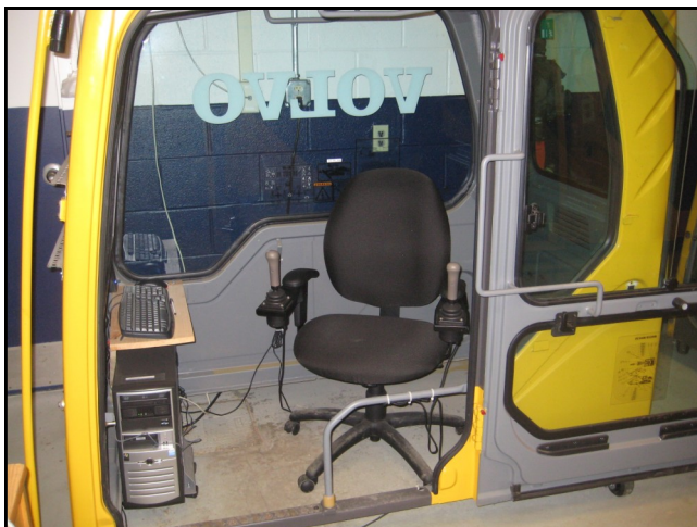
A closer look at Simlog's Hydraulic Excavator Personal Simulator with Original Equipment (OEM) joysticks mounted to an office chair inside a real excavator cab.
