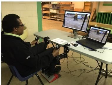
Hydraulic Excavator Personal Simulator Portable Station
