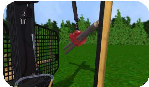
Loading logs into the forwarder's cradle from multiple log piles
